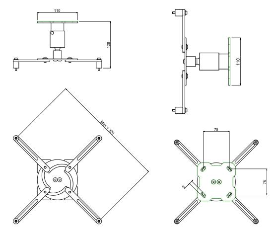
Including mounting material for connecting projector (M3, M4, M5, M6)
