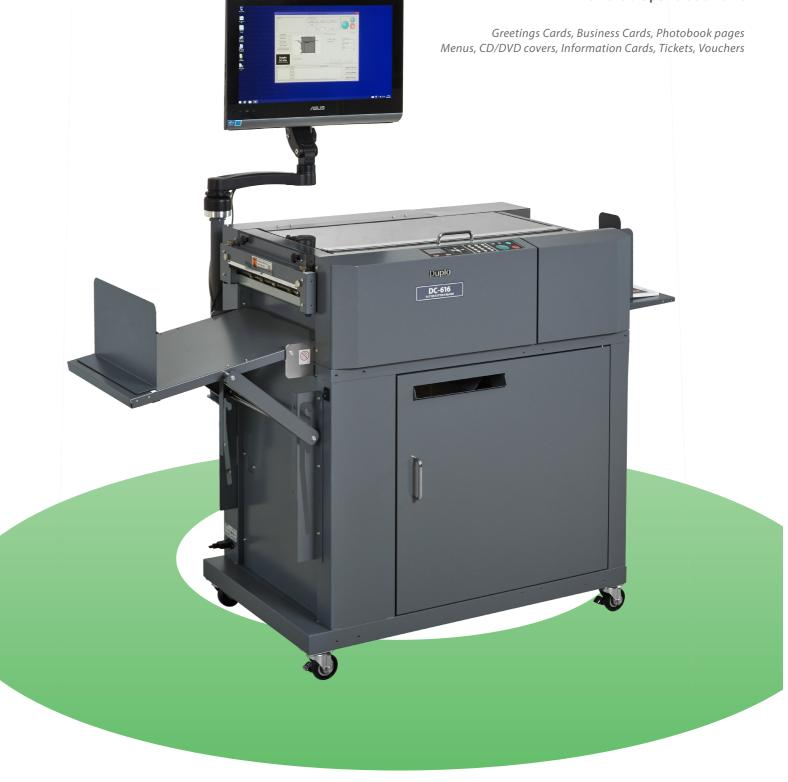
The DC-616PRO provides the shortrun on-demand digital printer, multifunction finishing in one compact, easy to use solution. It cuts, creases and perforates printed sheets, producing finished applications in a single pass.
