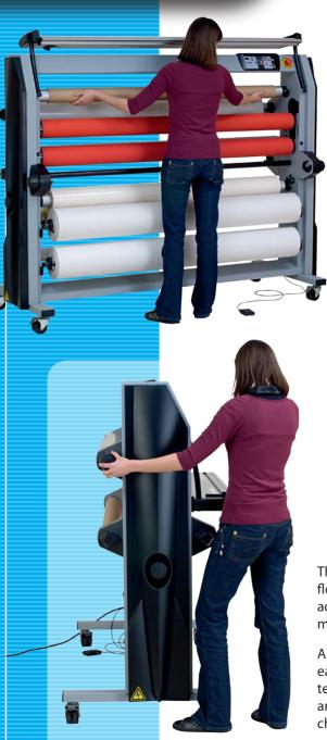
With our new even lighter self-blocking roll-shafts, you will save time while changing film. No tools are required unlike systems using locking rings or pivoting shafts needing a large space behind the machine.
