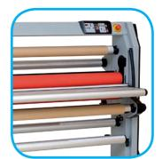
5 roll-shafts and one unwinding shaft delivered with the machine.
