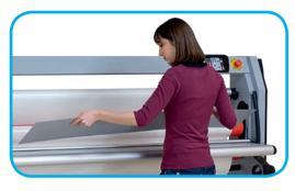
The machine is delivered with a metal feeding tray in order to reduce material waste and to save time when installing the film on the machine.
